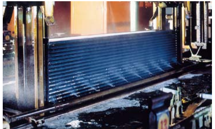
The Black Chrome Absorber - Solahart use a universally accepted method for absorber finishes - electroplating
