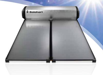
The double ceramic lined tank has a protective sacrificial anode and the Free Heat models feature additional anode protection. The tank is equipped with an electric booster, alternatively an inline gas booster is available.
