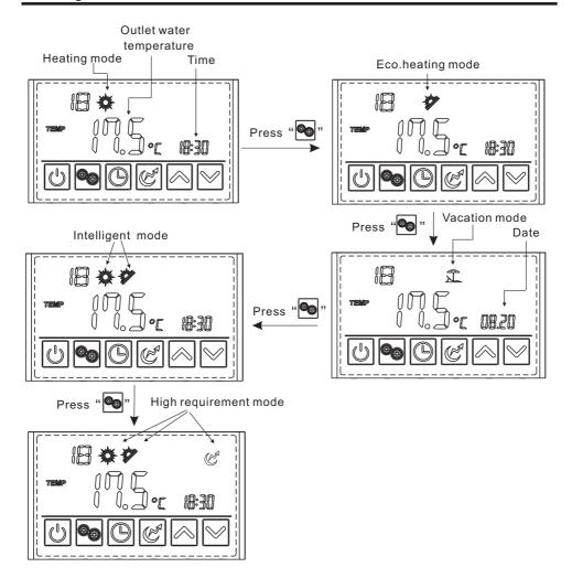
5.2.3 Target temperature checking and setting
