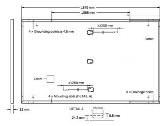
Fig. 1: External dimensions and components for Solahart415S3
