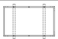
Fig 3. Bolt installation for 60cell
