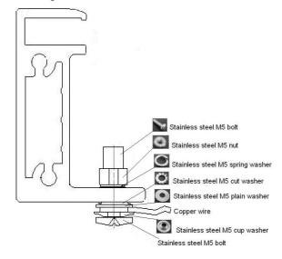
Fig. 15 Grounding the aluminum frame with copper wire
