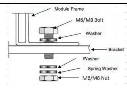
Fig. 7 Diagram of the bolt installation process
