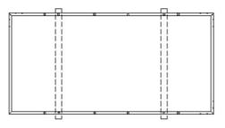
Fig 5. Internal four-hole bolt installation for 72cell
