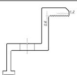
Fig. 11 Schematic cross section of the fringe clamp
