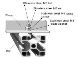
Fig. 12 Schematic diagram of the fringe clamp
