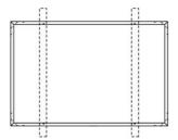
Fig 2. Bolt installation for 54cell
