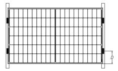
Fig. 9 Rails overlapping the short-side frame
