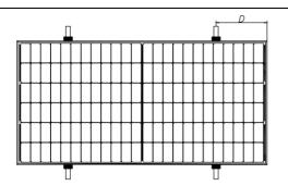
Fig. 8 Rails overlapping the long-side frame
