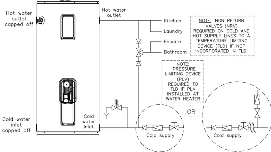
**Two Temperature Zones Using Temperature Limiting Device Hot Water Outlet – E6X Series**
